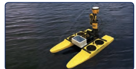
HyDrone™ ASV with Trimble SPS 585 and TSC3
